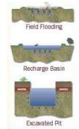
is applied and recharged. Monitoring wells would be installed to track changes in groundwater elevation and groundwater quality in response to percolation of surface water into the groundwater aquifer.
